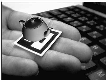
Fig. 3.1: Augmented Reality: A virtual object, i.e., a teapot is visually augmented to the real environment.
