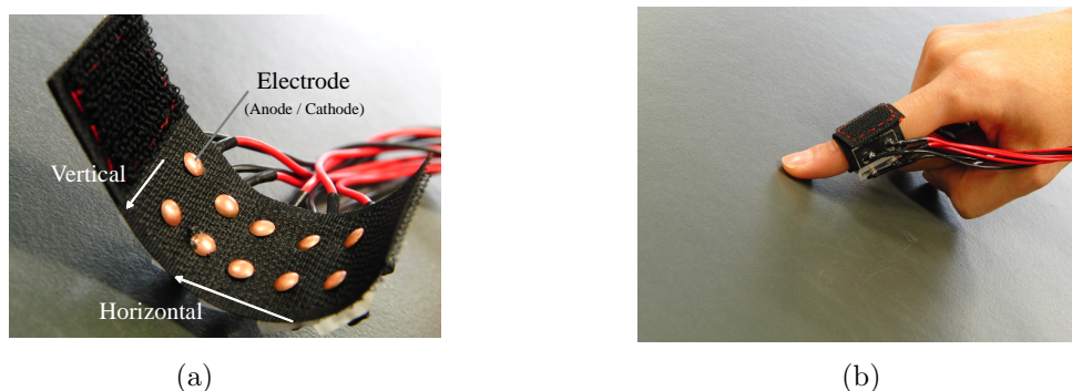
Fig. 4.9: Developed electrodes array: (a) Electrodes structure (b) Appearance of the use.
