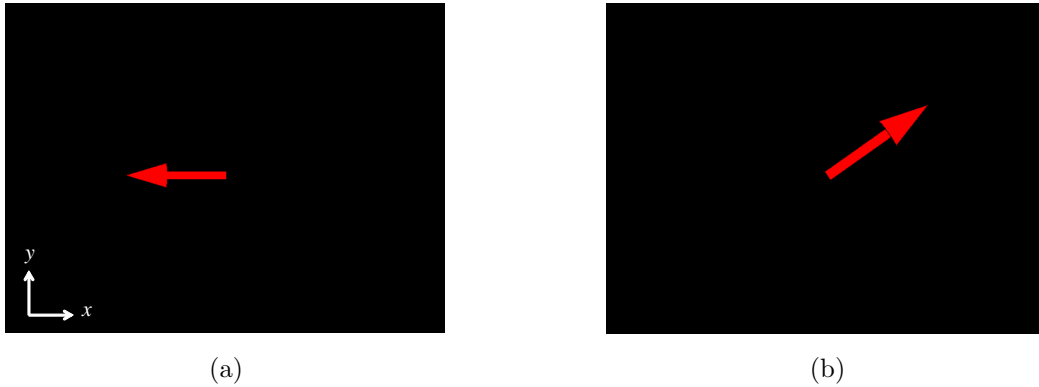
Fig. 6.13: Visual effect of force vector: (a) In case of (F_x, F_y, F_z) = (-1, 0, 0) . (b) In case of (F_x, F_y, F_z) = (1, 1, 0) .
